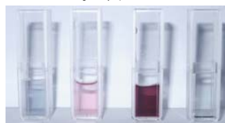
Fig. 4: Different particle types (from the left to the right): Nanoshells (IBMT) - Nanorods - Nanospheres - Nanoshells (commercial)
